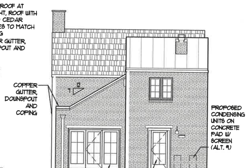
3 PROPOSED CARRIAGE HOUSE NORTH ELEVATION SCALE: 3/32" = 1'-0"
