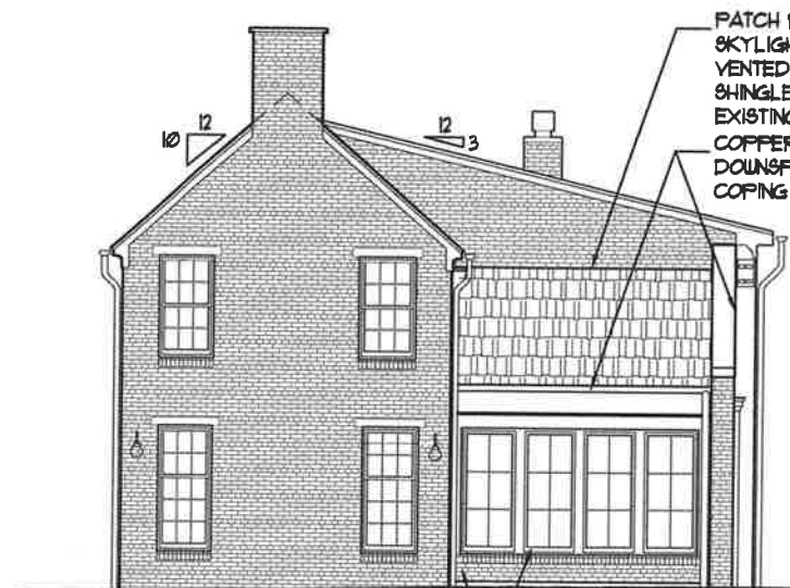
2 PROPOSED CARRIAGE HOUSE EAST ELEVATION SCALE: 3/32" = 1'-0"
