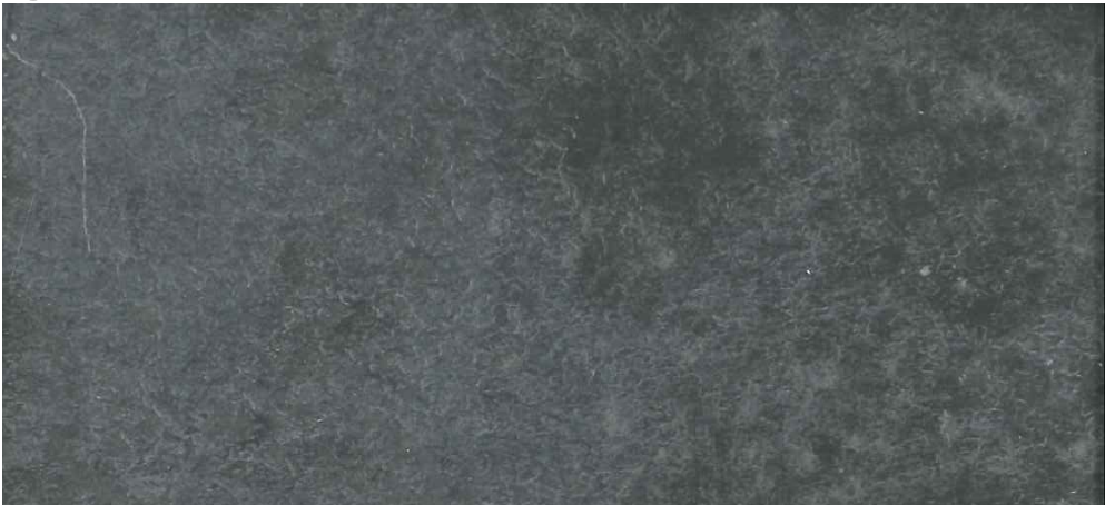
5 STONE SILL & WATERTABLE (AT BRICK): DARK GREY STONE
